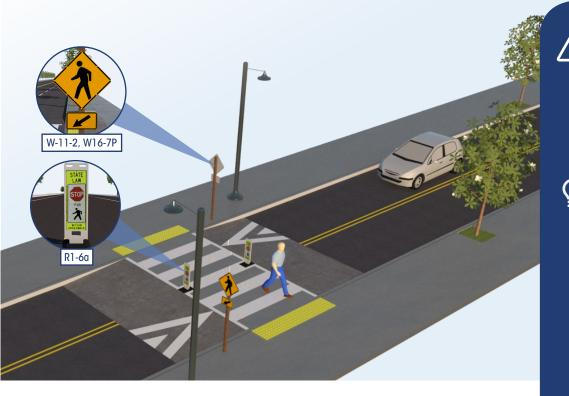
Raised crosswalks are ramped speed tables spanning the entire width of the roadway, often placed at midblock crossing locations. The crosswalk is demarcated with paint and/or special paving materials. These crosswalks act as traffic-calming measures that allow the pedestrian to cross at grade with the sidewalk.
